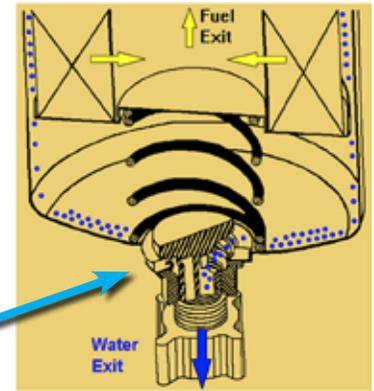
Fuel return line = water automatically put back into tank = longer engine life
